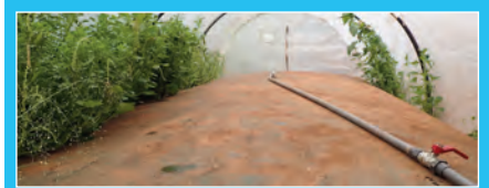
This is the fermentation bag, the pipe takes the biogas produced to the cooker; below, cooking on gas instead of fire
